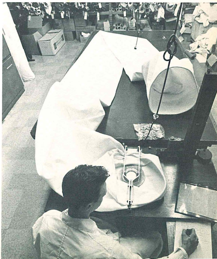
Air flow permeability is tested on 30 foot long fabric filter tubes at Criswell Division.
